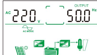
4) Battery working mode (Has PV input but no mains input, only the PV charge the battery)
